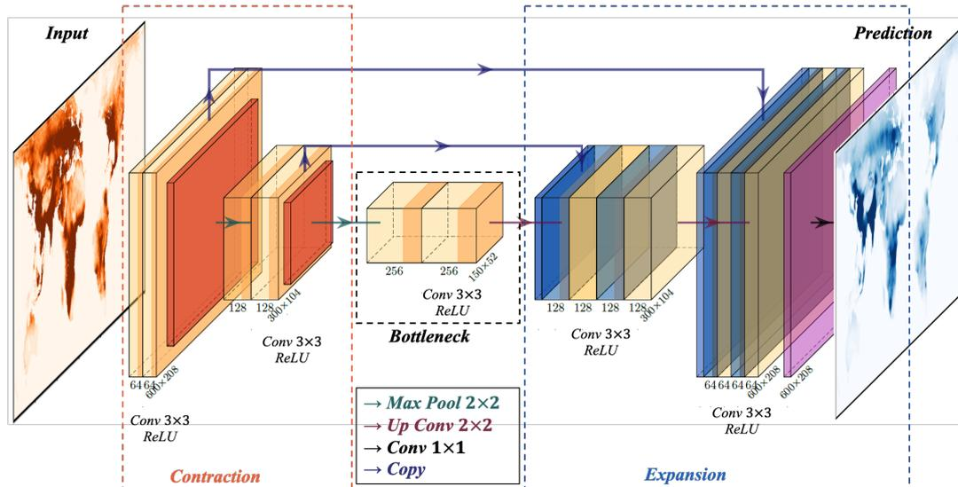
Figure 1. Architecture of the U-Net model
