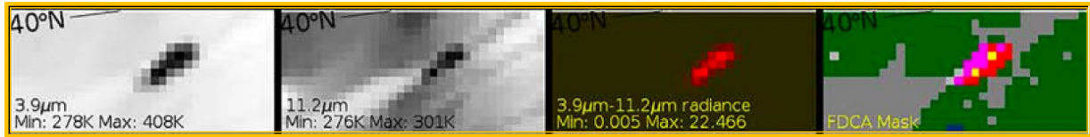
Figure 4: An illustrative example of the binary burning area data[30]. Left to right: GOES-R ABI at 3.9 and 11.2 \mu\text{m} bands, radiance difference between the 3.9 and 11.2 \mu\text{m} bands, and the Fire Detection and Characterization Algorithm (FDCA) data mask for Camp Fire, 2018.
